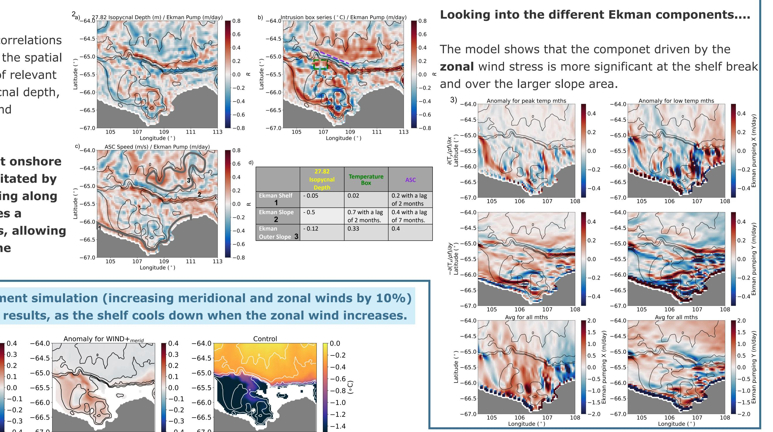
The Easterlies experiment simulation (increasing meridional and zonal winds by 10%) is consistent with our results, as the shelf cools down when the zonal wind increases.
