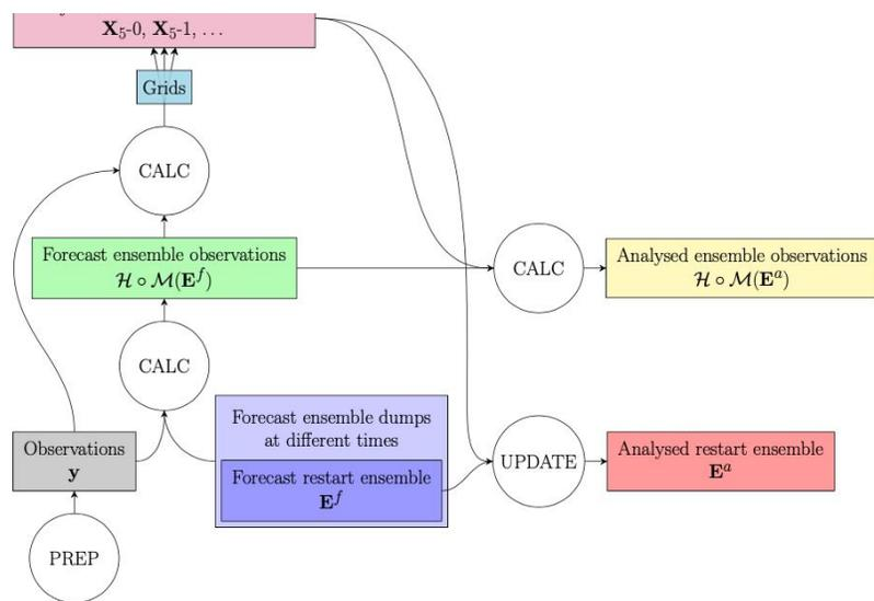
Figure 2.1: The principle diagram of EnKF-C workflow.
