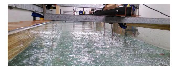
Experiments using Froude scaling (Pi Theorem) to replicate in controlled environment field observations and test mathematical models
